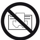
**“DO NOT COVER”, which acts as a reminder for the user. It is recommended that the air contacts all the surfaces of the heater.**
