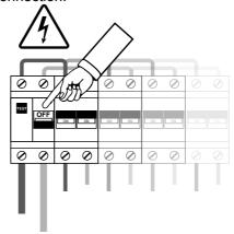
Connect the power supply cable to the terminals  ${\bf L}$  and  ${\bf N}$  of the Power Monitor. Remember to disconnect the power supply from the circuit breaker where the Power Monitor will be connected.
