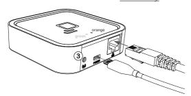
Once the Gateway is connected to the Internet and registered in the web portal, the devices must be paired to it. To do this, put the Gateway in discovery status press the **Link** button for 3 seconds.
