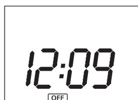
To return the heater to a heating mode, press the **MODE** button to choose programme mode (**AUTO**) or **MANUAL** mode
