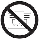
**Warning: in order to avoid over heating the unit, do not cover the heaters. This symbol “DO NOT COVER”, is placed on the heater as a reminder to the user.**
